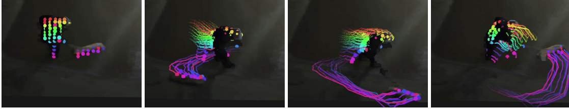
Figure 2: Example 3D point tracks reconstructed by 3DSPA for a generated video of a man mopping a floor in the VideoPhy-2 dataset (Bansal et al., 2025). This video has a good human rating and was reconstructed pretty well by our model.
