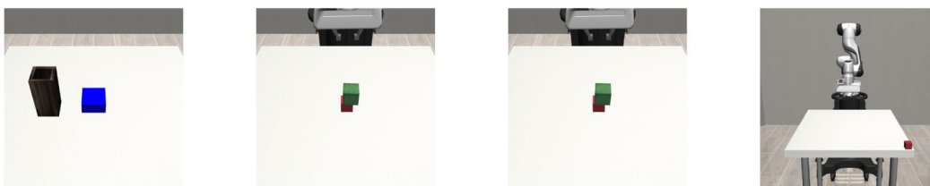
Figure 6: Example scenes corresponding to each constraint domain (left to right): (a) Impossible Placement : attempting to fit the blue block into the brown box; (b) Occlusion/Support Issues : picking up the red block beneath another; (c) Stability Constraints : lifting the unstable green block from the top of a stack; (d) Reachability and Access Constraints : grasping a block placed at the very edge of the workspace.
