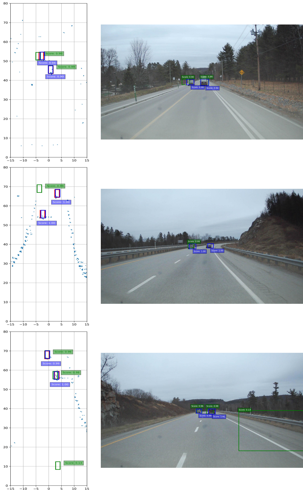
Figure 9: Detection results of FFT-RadNet (green) and our proposed network “frozen_enc”(blue). The bounding box prediction of FFT-RadNet is displaced w.r.t the ground truth bounding box (red), whereas the “frozen_enc” prediction aligns well with the ground truth. Confidence score equals 0.1. Left: Bounding boxes in Cartesian coordinates displayed on lidar point clouds. Right: Bounding boxes projected on image.
