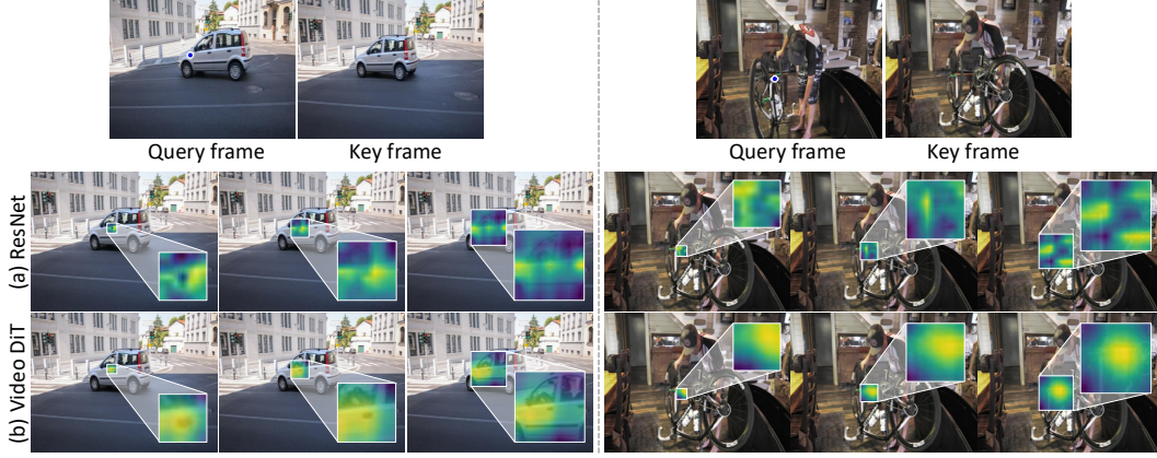
Figure 2: Visualization of pyramid local costmaps. For the query point on the left images, we compute feature similarity between the query point and key points from each image over multiple feature resolutions and visualize the cost map. (a) ResNet features often become noisy when the target point is on textureless region or moves outside a local window. (b) Video DiT features, on the other hand, clearly highlight the direction of the true target point.
