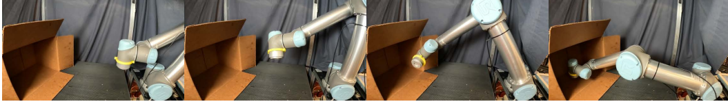
Figure 4: Demonstration of a motion plan on hardware. The goal is to reach into the box without making contact.
