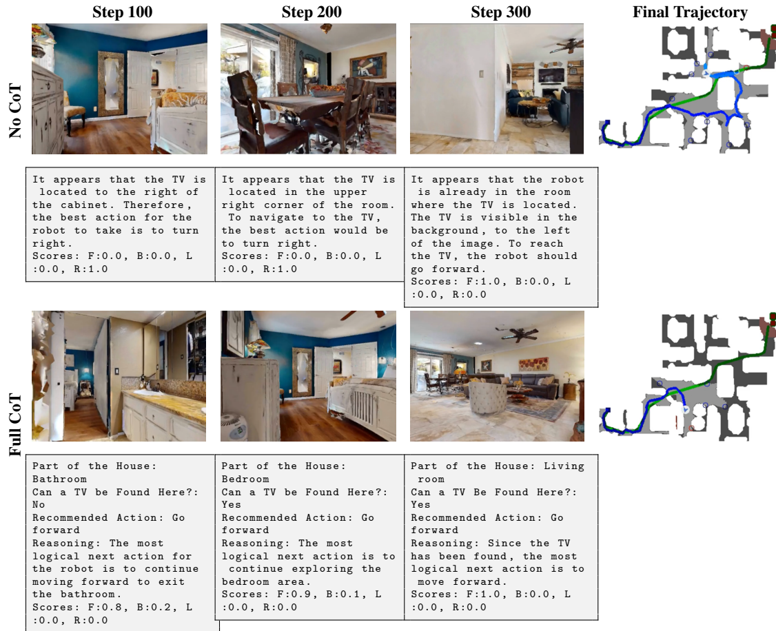
Figure 4: Qualitative analysis of navigation with and without our full CoT framework. The agent’s view and the VLM’s reasoning are shown at various timesteps. The top row (No CoT) displays an agent with basic reasoning that wanders aimlessly and fails to locate the target. The bottom row (Full CoT) illustrates how a structured, step-by-step reasoning process (such as identifying a bathroom, realizing a TV is not there, and choosing to leave) results in a more intelligent exploration strategy and a direct, successful path. This comparison underscores the crucial role of CoT in achieving more effective and intelligent navigation.
