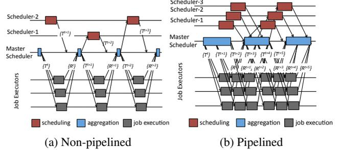
Figure 3: **Dynamic Engine** pipelining: (a) Non-pipelined execution: network latency dominates; (b) Pipelining overlaps networking and computation.
