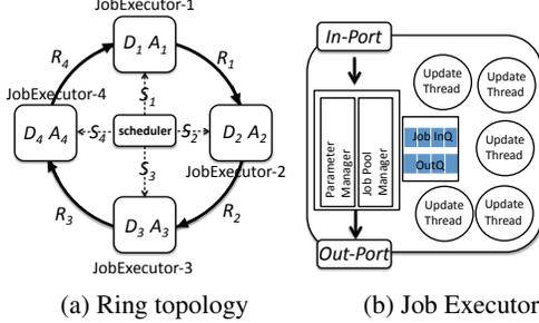
Figure 2: **Static Engine**: (a) Parameters  $A_p$  and intermediate results  $R_p$  are exchanged over a ring topology. (b) **Job Executor** architecture: the **Parameter Manager** and a job pool manager receive and dispatch jobs to executor threads; results  $R_p$  are immediately forwarded without waiting for other jobs to complete.
