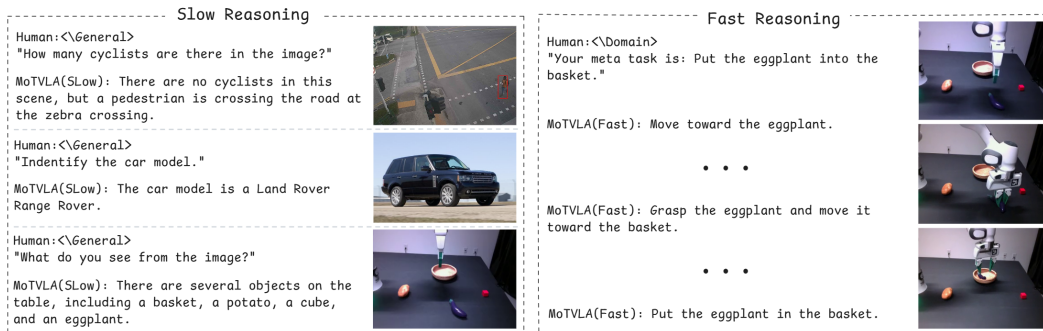
Figure 5: A concrete example of fast and slow reasoning during inference. When asked a general question, the generalist performs slow reasoning and provides a detailed verbal response. When a task-execution prompt is issued, the domain expert performs fast reasoning to generate decomposed intermediate motions for action execution.
