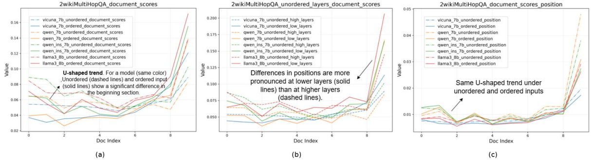
Figure 3: Relationship between attention weight scores and document positions on the 2wikiMultiHopQA dataset. Figure (a) shows comparison between ordered and unordered inputs(horizontal). Figure (b) compares different layers under unordered inputs(vertical).Figure (c) compares extracted position scores under ordered and unordered.
