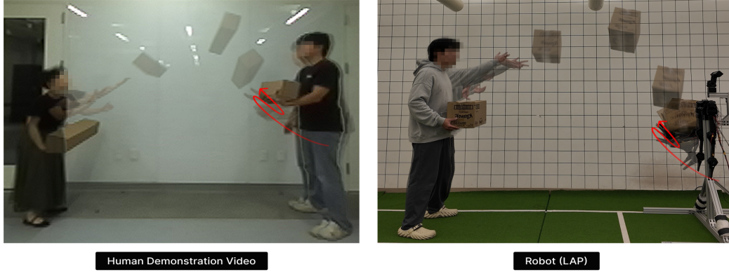
Figure 3: Impact-aware retreat trajectory for box catching motion learned with the Latent Adaptive Planner (LAP). The left panel shows a human demonstration where the subject absorbs impact by yielding their arm along the trajectory of the incoming box before returning to the nominal pose. The right panel shows the robot reproducing this compliant motion using LAP. The red curves indicate the impact-aware retreat trajectory that minimizes energy consumption during dynamic interaction.
