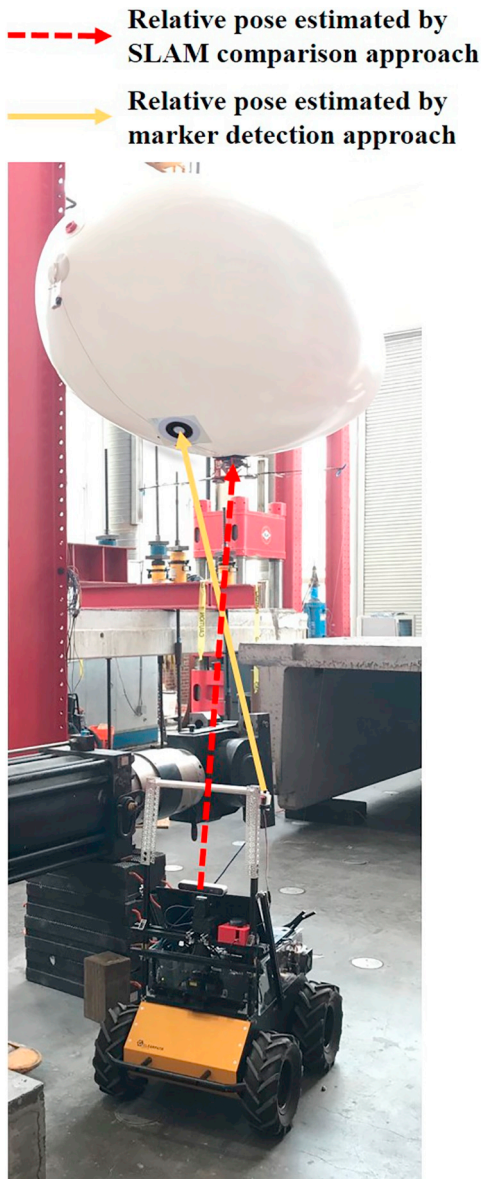
Fig. 25. Relative pose estimated by SLAM comparison and marker detection approaches.
