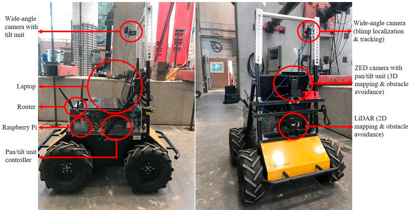
Fig. 5. UGV's hardware description.
