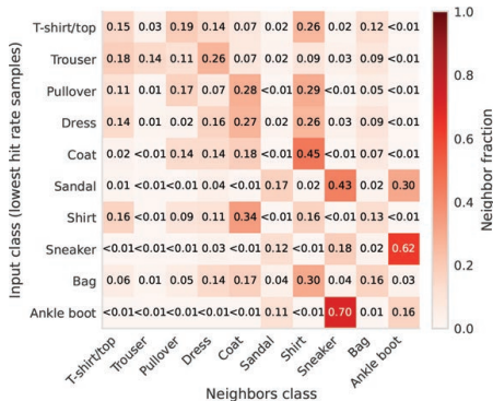
Figure 11: Neighbor confusion matrix (FashionMNIST) inputs with the lowest neighbor label hit rate (worst 5k samples). Each row corresponds to an input class and each column to a neighbor class; entry (i, j) gives, averaged over low-hit inputs of class i , the fraction of their k -NN that belong to class j .
