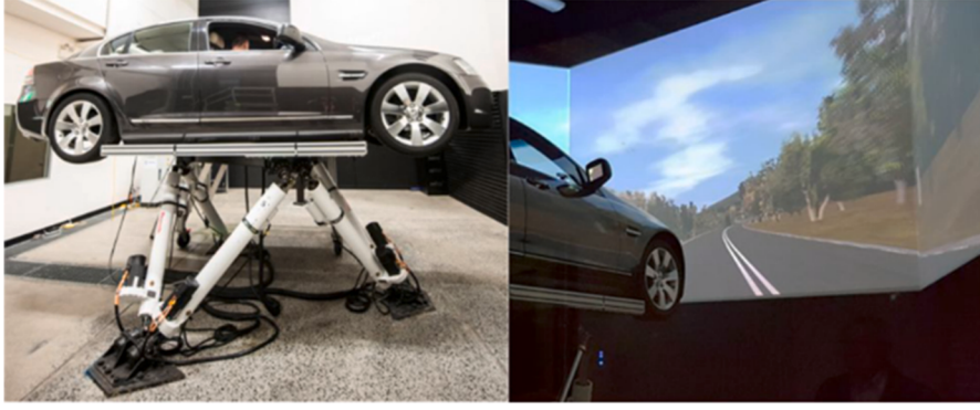
Fig. 1. CARRS-Q's driving simulator was used to collect data. The simulator consists of a front view (180 degrees), rear view mirror image, real cabin, audio system to simulate the driving environment and a six degree of freedom motion platform, as well as the SCANeR™ studio and FaceLAB™ remote video eye tracker.
