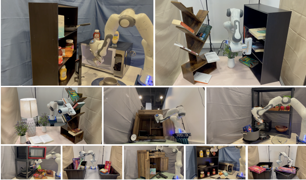
Figure C.1: Neural Motion Planning at Scale in the Real World Our approach enables a single, generalist neural network policy to solve motion planning problems across diverse setups; Neural MP can generate collision free motions for a wide array of unseen tasks significantly faster and with higher success than traditional as well as learning-based motion planning approaches.
