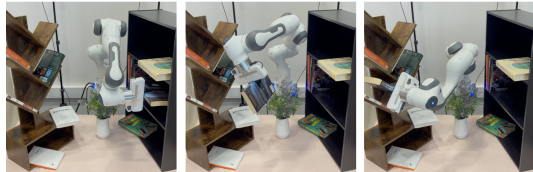
(c) Our policy has not been trained on this bookcase, yet it is able to insert the book into the correct location.
