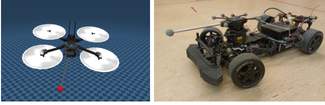
Fig. 2: Experimental platforms used to validate the proposed method: (i) drone with rope attached payload trajectory tracking, (ii) real-world autonomous F1TENTH [36] racing.
