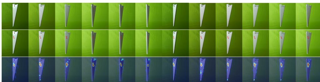
Figure 25: Similarity scores for the data subset bracket. The first row represents the input, and we circle the anomaly regions in the second row. The last row presents the segmentation results from AnomalyCLIP.
