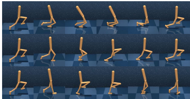
Figure 10: The behaviors generated by AlignDiff when only adjusting the left-right leg preference attribute. From the first row to the last row, they respectively represent attribute strength values of [0.9, 0.5, 0.1].
