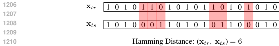
1211 Figure 7: Hamming distance between a training set individual \mathbf{x}_{tr} and a new individual \mathbf{x}_{ts} .
