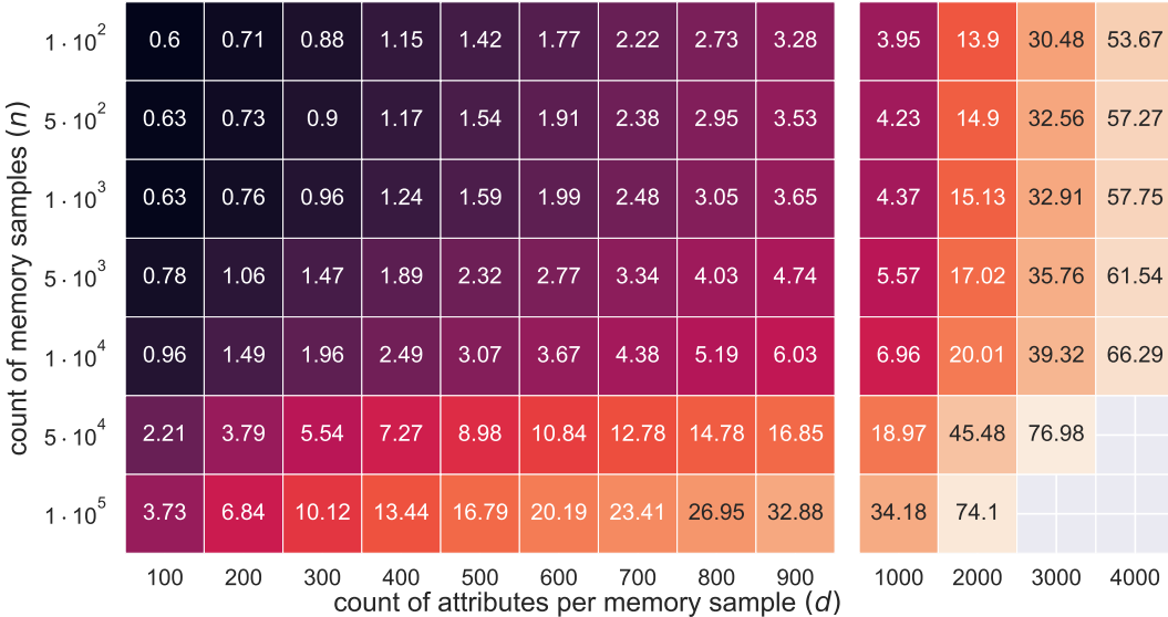
Figure A.5: Memory footprints of Hopular in gibibytes (GiB) measured on an artificially generated dataset. Missing entries denote settings which do not fit on an NVIDIA A100 80GB GPU, i.e. run out of memory. Best viewed in color.
