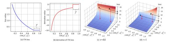
Figure 3: (a) and (b) are the curves of the ITA loss and its derivative, respectively. (c) and (d) are the 3D surface plots of our IAR loss with different  $\tau$ . The samples A and B have the same  $\text{sim}(\mathbf{p}_i^{k_1}, \mathbf{q}_j^{k_2})$ , but  $\text{sim}(\mathbf{p}_i^{k_1}, \mathbf{p}_j^{k_2})$  of A is smaller that of B. When  $\tau = 0.1$ , the IAR loss values of A and B are almost the same, but when  $\tau = 1$ , The loss value of A is much smaller than that of B.
