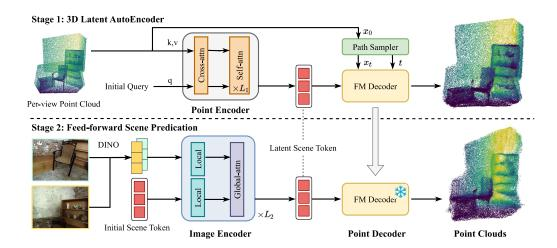
Figure 3: **Overview of NOVA3R. Stage 1:** a 3D point autoencoder encodes complete point clouds into latent scene tokens and decodes them with a flow-matching (FM) decoder. **Stage 2:** an image encoder with learnable scene tokens integrates multi-view information into a unified scene latent space, supervised by the FM loss with the Stage-1 decoder frozen. During **inference**, only the second stage pipeline is used to produce a complete, non-pixel-aligned point cloud.
