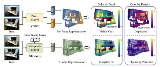
Figure 1: **NOVA3R** enables non–pixel-aligned reconstruction by learning a global scene representation from unposed images. Compared to pixel-aligned methods, NOVA3R recovers both visible and occluded regions and produces more physically plausible geometry with fewer duplicated structures.
