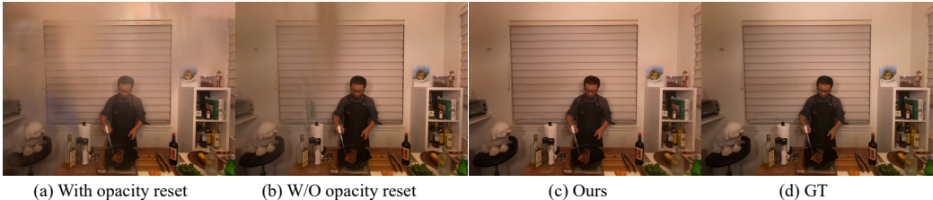
Figure 9: Importance Pruning Ablation Experiments: (a), (b), (c), and (d) show the rendered results of the our model with opacity reset every 3000 iterations, without opacity reset, with our importance pruning method, and the ground truth, respectively.
