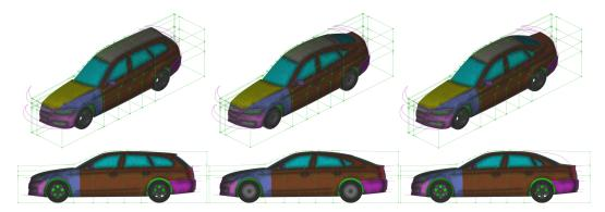
Figure 6: Three parametric models from DrivAerNet++. The green boxes represent the morphing boxes, and the purple curves illustrate the trajectories followed during the morphing of the car geometry. A total of 26 parameters were utilized to adjust and refine the car designs.
