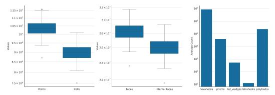
Figure 11: Mesh statistics for the DrivAerNet++ dataset. Left: distribution of points and cells; middle: distribution of faces and internal faces; right: average cell counts by type.
