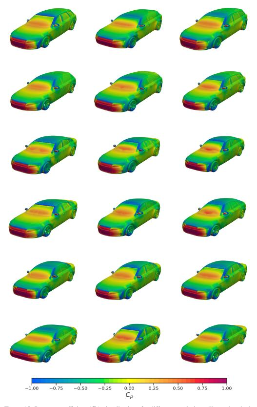
Figure 15: Pressure coefficient  $(C_p)$  visualizations for different car designs, illustrating the large variations in shape within the DrivAerNet++ dataset. The color indicates the pressure coefficient  $C_p$ , with values ranging from -1.00 to 1.00.
