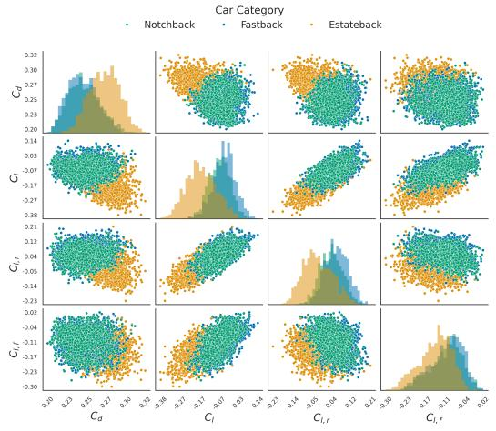
Figure 13: Pair plot showing the relationships between different aerodynamic coefficients ( $C_d$ ,  $C_l$ ,  $C_{l,r}$ , and  $C_{l,f}$ ) in the DrivAerNet++ dataset. The diagonal histograms represent the distribution of each coefficient, while the scatter plots show the pairwise correlations between the coefficients. The colors represent different configurations within the dataset, illustrating the diversity in aerodynamic performance.
