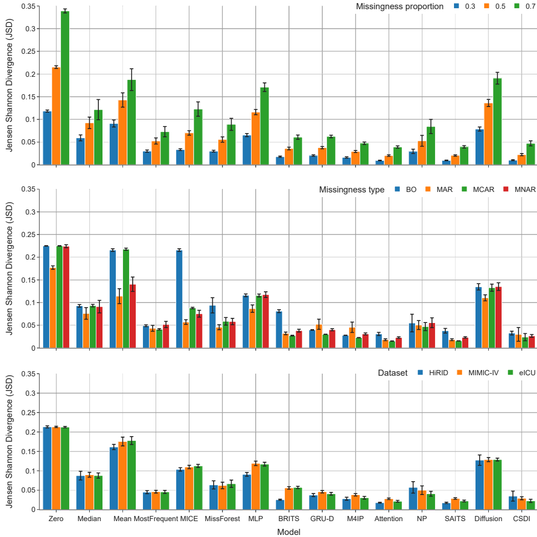
FIGURE 3: Performance in JSD across the selected imputation methods in three dimensions. Top: imputation methods separated by missingness proportion for MNAR. Middle: aggregated performance per missingness type. Bottom: aggregated performance for each dataset.
