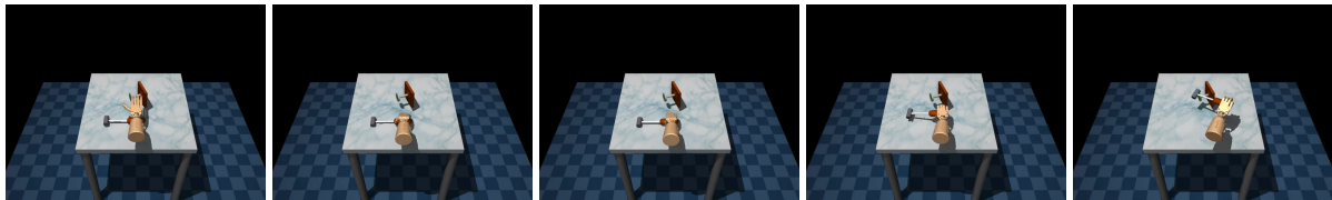
Figure 6. Visualization of a typical failure trajectory of the forward policy. Note that the hammer hits the nail but does not fully push the nail into the board.
