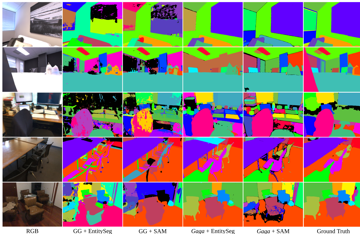
Figure 6: Qualitative results on Replica and ScanNet. Gaga consistently predicts more accurate segmentation masks. Gaussian Grouping often covers the same object with different masks (row 1, 3, 5), creating large empty regions (row 1, 2, 3), or misidentifying similar instances (row 4, 5).
