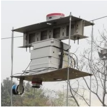
Figure 2: Portable robotic platform with Lidar, multispectral camera, GPS and IMU mounted.
