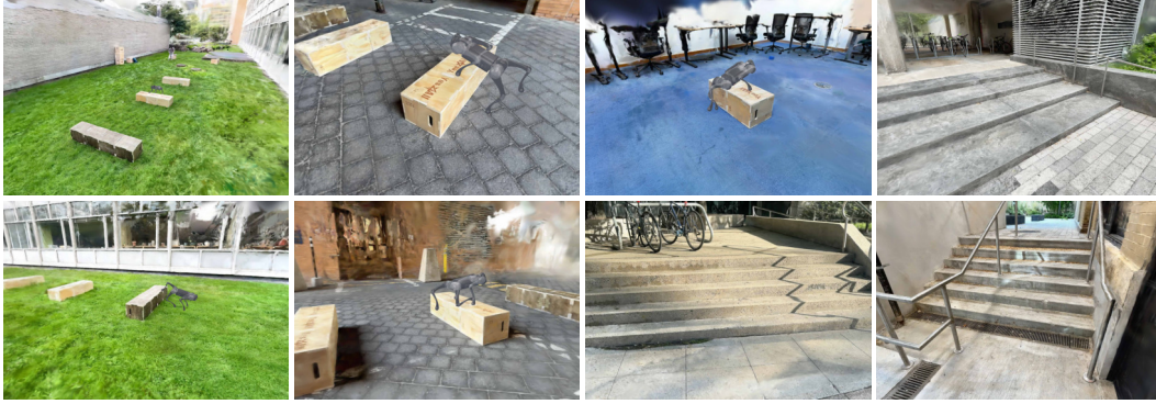
Figure 9: Rendered views of a subset of environments used for evaluation. Each scene is modeled using 3D Gaussian Splatting. The first-person view from the robot’s perspective is highly realistic.
