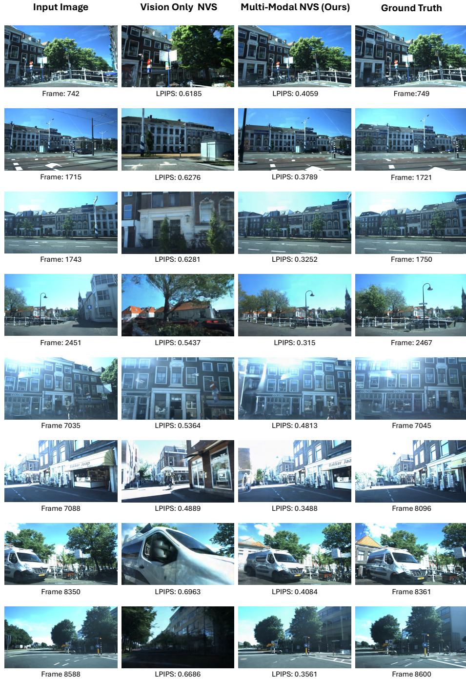
Figure 3: Qualitative comparison on single-image novel-view synthesis on the View-of-Delft dataset. From left to right, we show the input image, the novel view generated by GEN3C (Ren et al., 2025) using its default monocular depth estimator, MoGe (Wang et al., 2025), the novel view generated by GEN3C when replacing monocular depth with our sparse range-sensor depth reconstruction module, and the ground-truth target view. For each generated view, we report LPIPS with respect to the ground truth (lower is better). Across all examples, our depth reconstruction yields consistently lower LPIPS and improved geometric alignment, underscoring the importance of reliable geometry for diffusion-based rendering from single-view inputs.
