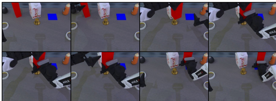
(c) Handover block: With the left arm, grab the red block, pass it to the right, and set it on the blue pad.
