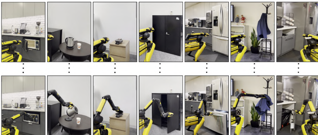
Figure 1: Glimpse of the diverse robot manipulation capabilities across physical office and kitchen scenes enabled by Track2Act . We learn to predict point tracks from web videos for learning interaction plans that can be used for inferring robot actions in unseen scenarios. This enables a common goal-conditioned policy to perform everyday tasks like closing microwaves, pulling out drawers, flipping open toasters, pouring from jars etc. Columns show first/last images of policy rollouts.
