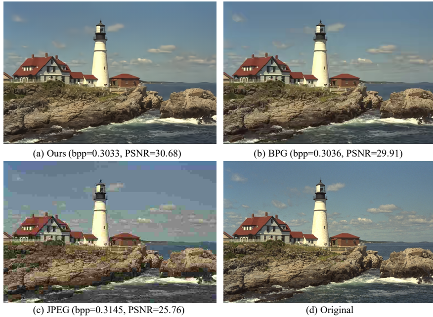
Figure 15: At similar bit rates, our combined method provides the highest visual quality on the Kodak 21 image. BPG shows more “classical” compression artifacts, e.g. , ringing around the edge of the lighthouse.
