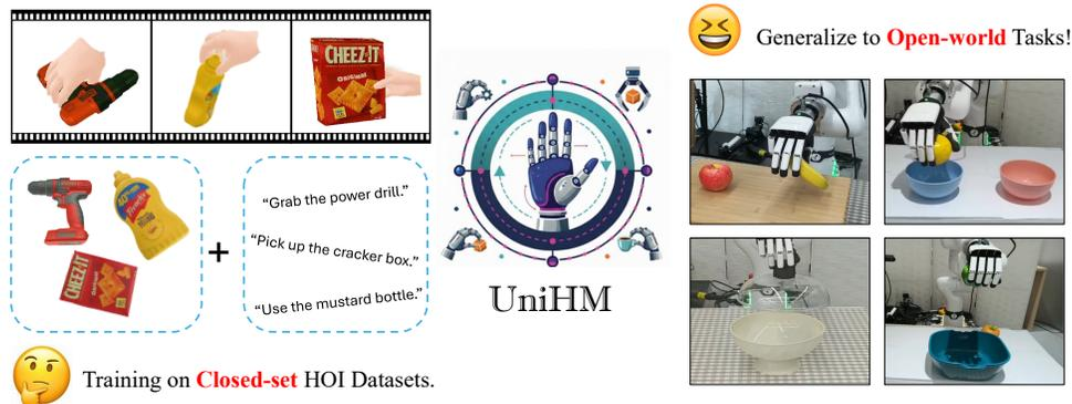
Figure 1: **Overview.** We introduce UniHM, the first unified hand-manipulation framework conditioned on free-form language. UniHM is trained solely on closed-set HOI datasets to follow target trajectories and execute physically feasible interactions, and generalizes to open-world tasks in real-world interactions.
