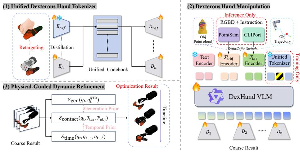
Figure 2: **Pipeline.** UniHM converts open-vocabulary instructions and RGB-D inputs into executable dexterous-hand trajectories via three stages: (1) morphology-agnostic motion tokenization; (2) language-guided generation that fuses text, perception, and token history to produce manipulation token sequences; and (3) physics-aware decoding with smoothness/contact priors for feasible, stable execution.
