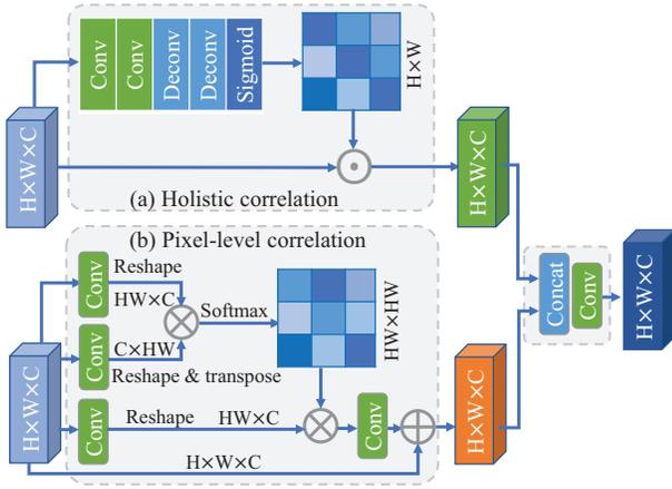
Figure 2: Architecture of the proposed Fine-grained Aware Network (FANet). It consists of a holistic correlation module and a pixel-level correlation module. The input and output are a  $H \times W \times C$  feature map,  $\odot$  denotes the broadcast element-wise multiplication,  $\otimes$  denotes the batch matrix multiplication, and  $\oplus$  is the broadcast element-wise addition.
