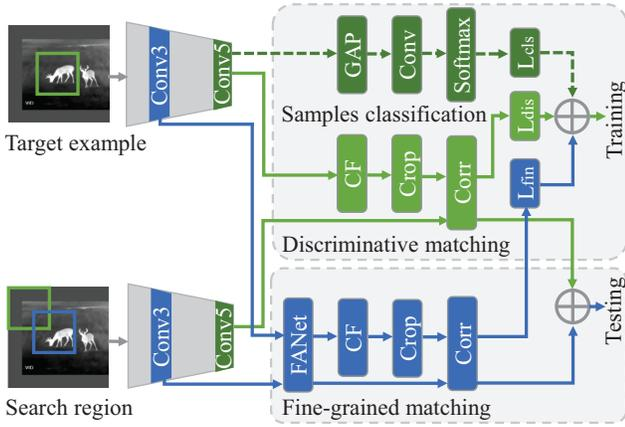
Figure 1: Architecture of the proposed Multi-task Matching Network (MMNet). It comprises a shared feature extracted network, a classification branch, a discriminative matching branch, and a fine-grained matching branch. In this figure, every box denotes a network layer or a subnetwork. Conv, GAP, CF, Corr, and FANet denote the convolution, global average pooling, correlation filter, cross-correlation, and fine-grained aware network (see Fig. 2), respectively.
