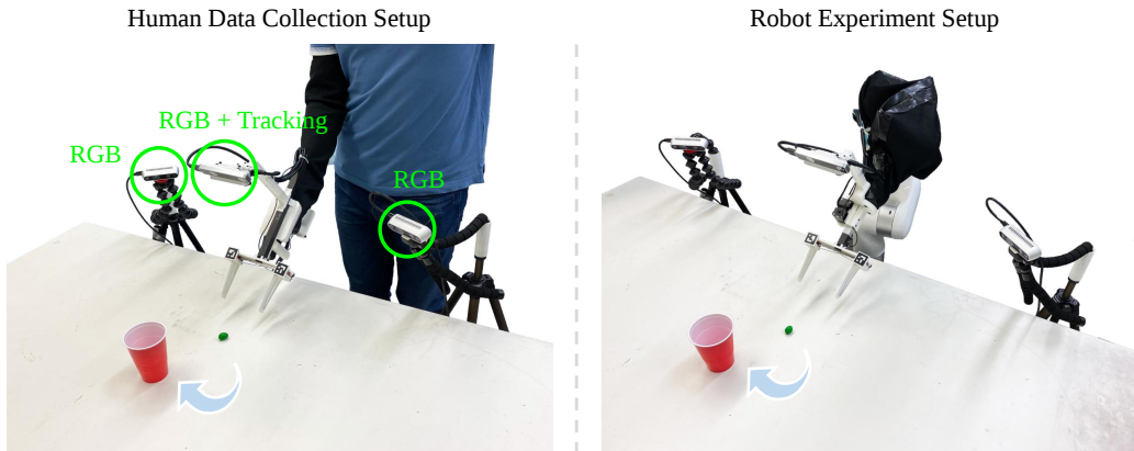
Figure 13: Data collection and robot experiment setup. During data collection, a human demonstrator performs the task using a modified robot gripper. In the robot experiment, the robot executes the tasks with the same setup.
