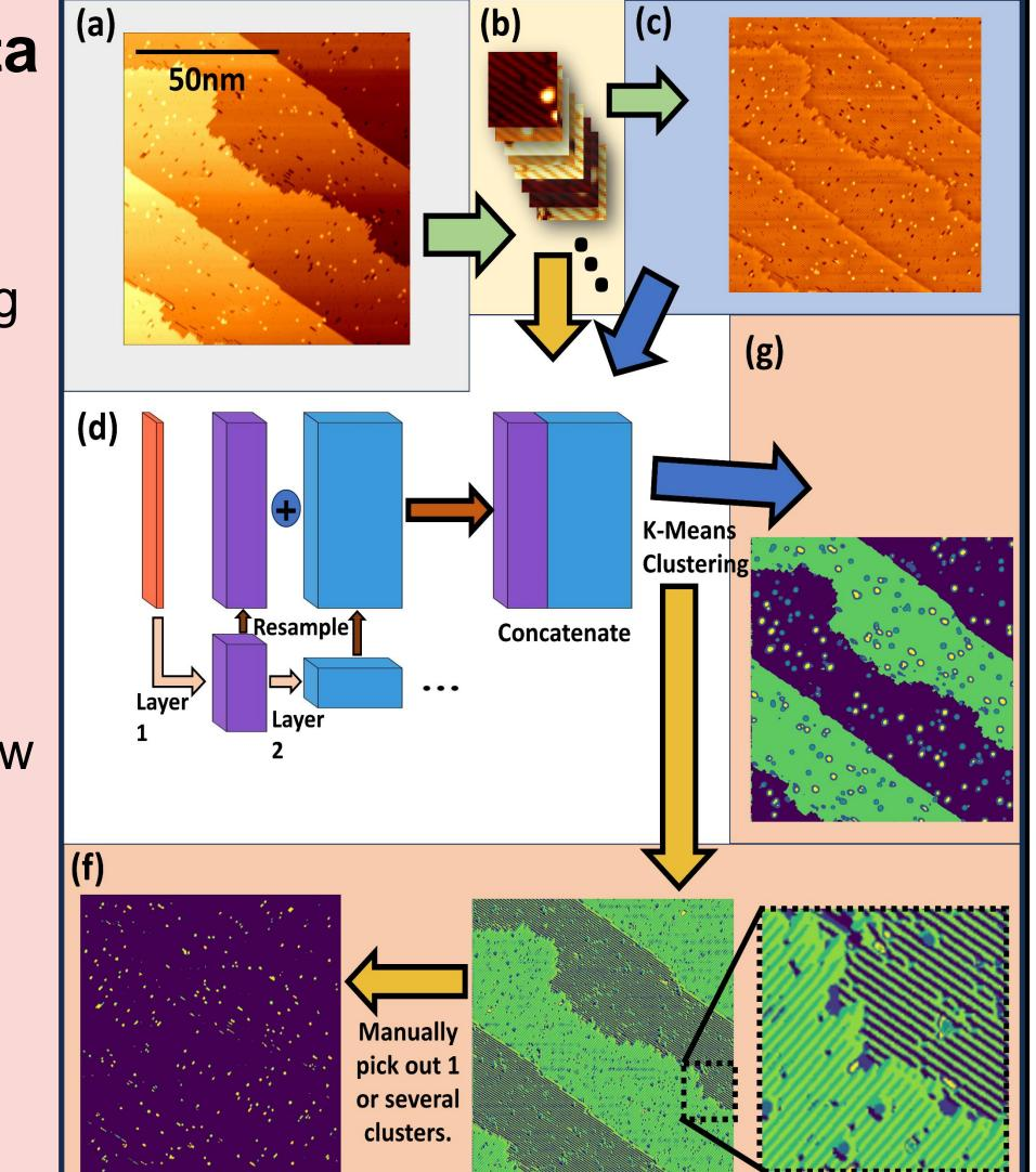
Each pixel in an image represents the height of the density of electron states at that point. We can measure either the filled or empty states, producing 2 channels.
