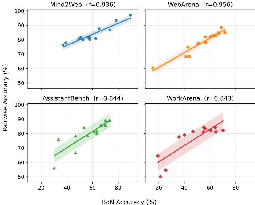
Figure 4: Correlation between BoN and Pairwise Acc across web benchmarks. Each scatter point corresponds to a PRM. We report the correlation coefficient r for each environment. While the two metrics are strongly correlated across all environments, BoN exhibits higher variance and provides finer-grained discrimination among models, particularly in complex web environments.
