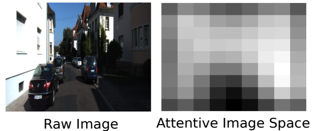
Fig. 2: Feature to Descriptor: We obtain attentive features from our AttentionNet output heads, which are further overlayed by the baseline feature detectors. This overlaying of baseline feature detectors on our attentive image space refines the outliers.
