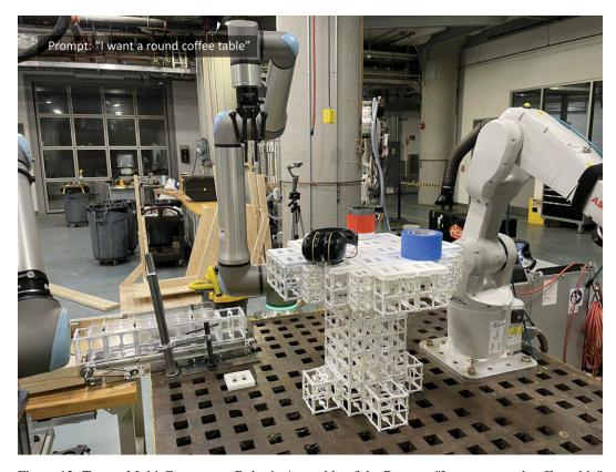
Figure 13: Text to Multi-Component Robotic Assembly of the Prompt: "I want a round coffee table"
