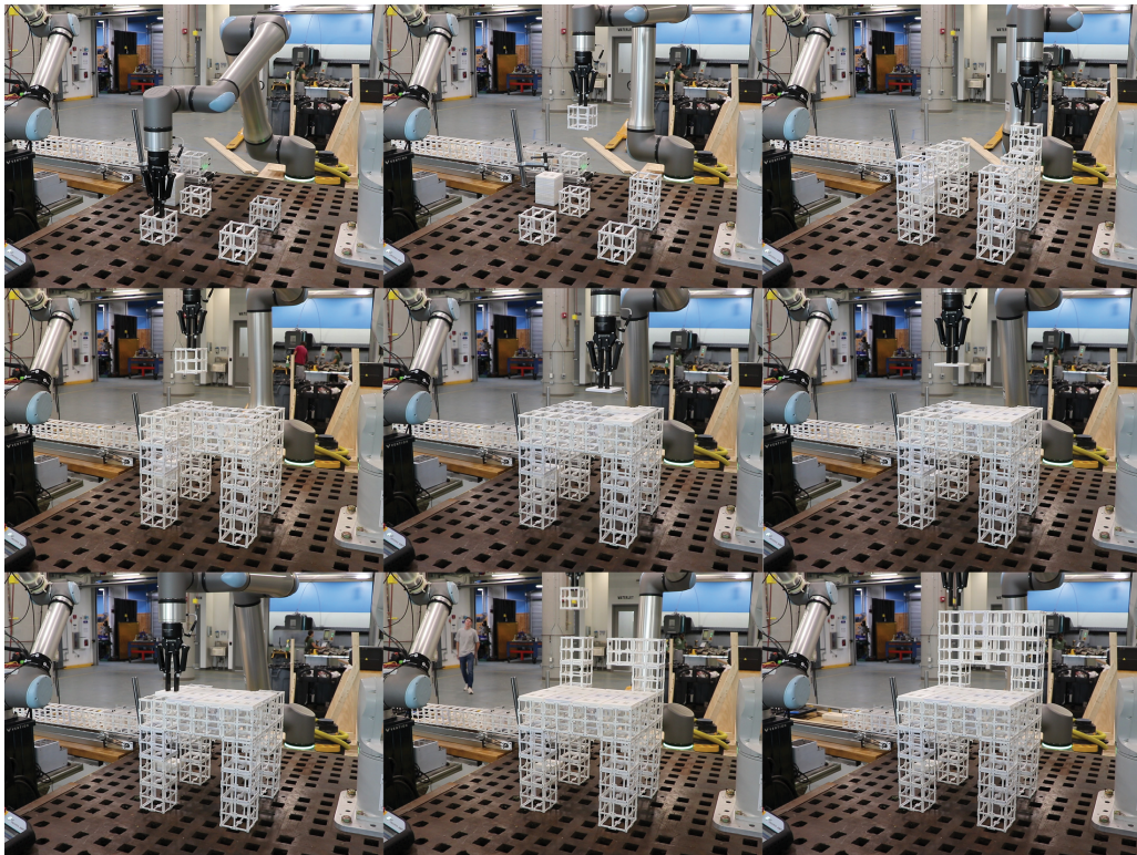
Figure 9: The robotic assembly process of the prompt: "Make me a chair", "I want panels on the seat"
