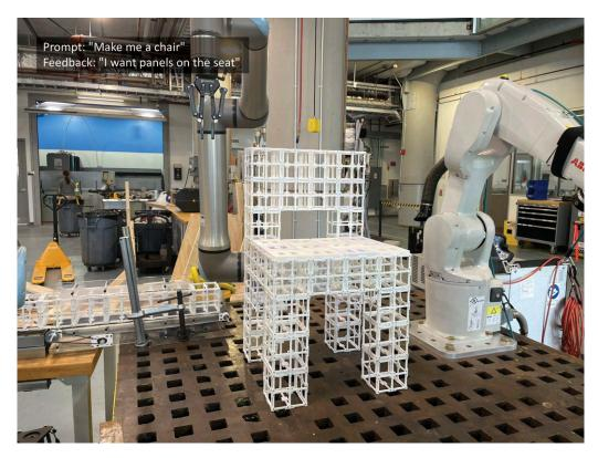
Figure 8: Text to Multi-Component Robotic Assembly of the Prompt: "Make me a chair", "I want panels on the seat"
