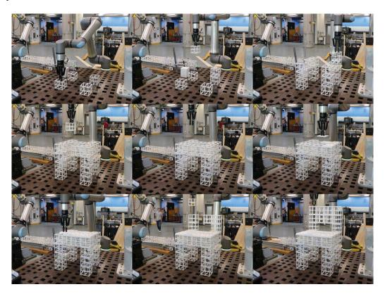
Figure 9: The robotic assembly of the prompt: "Make me a chair", "I want panels on the seat"
