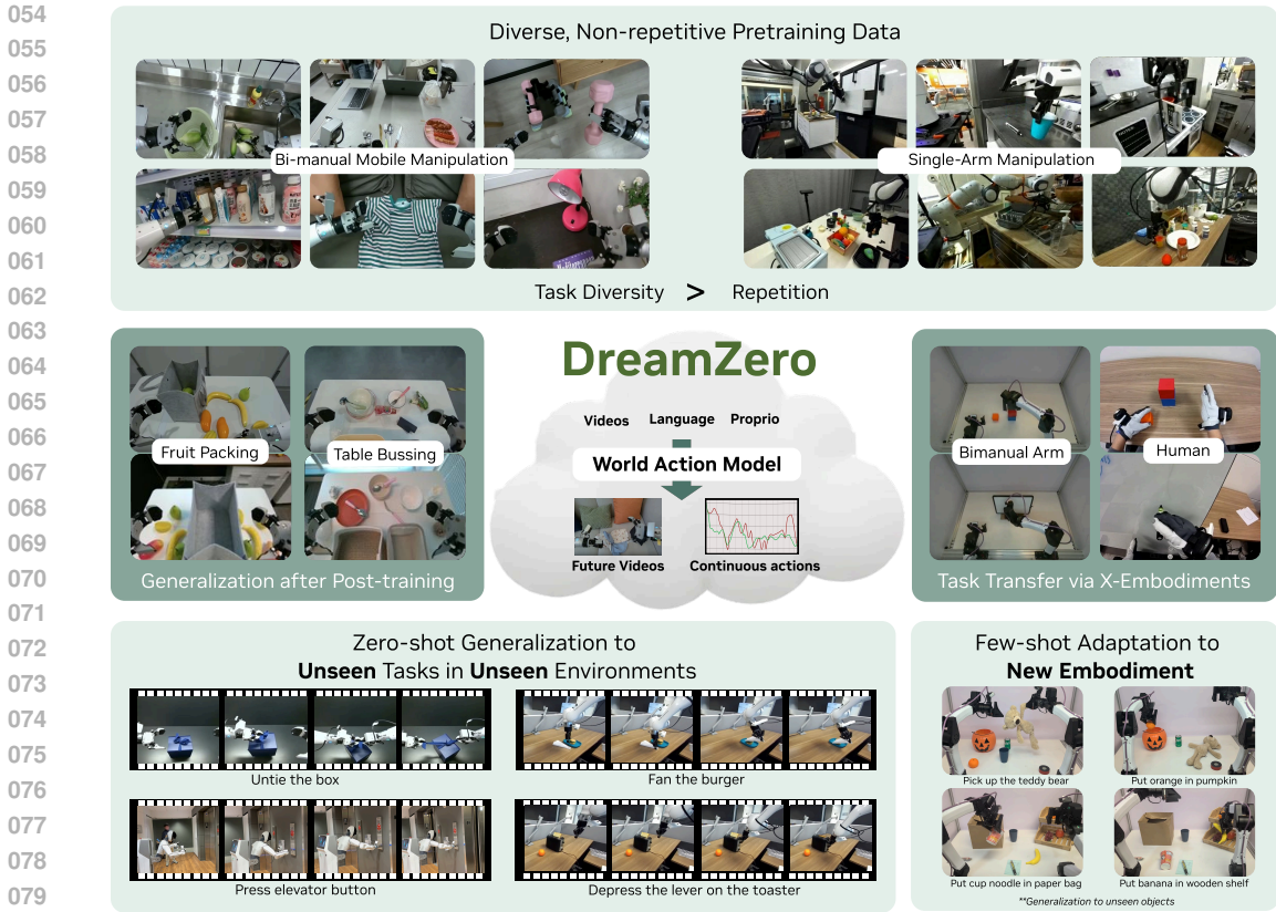
Figure 1: Overview. World Action Models (WAMs) inherit world physics priors that enable effective learning from diverse, non-repetitive data, open-world generalization, cross-embodiment learning from video-only data, and efficient adaptation to new robots.
