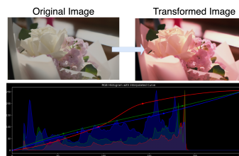
Figure 2: Example of image modifications using randomly generated tone curves. Independent curves are applied to the red, green, and blue channels, producing diverse color and contrast changes. The transformations simulate variations introduced by ITM algorithms and are used to elicit human aesthetic preferences during subjective evaluation.
