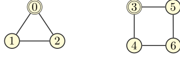
Figure 2: Two structurally different graph nodes (0 and 3) get the same color at every coloring round.
