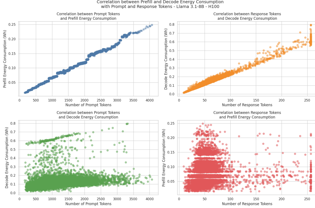
Figure 4: Correlation between token lengths and GPU energy consumption in prefill and decode phases.
