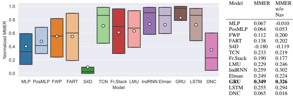
Figure 3: (Left) A summary comparison of baselines aggregated over all environments. We normalize the MMER such that 0 denotes the worst trial and 1 denotes the best trial for a specific environment. We report the interquartile range (box), median (horizontal line), and mean (dot) normalized MMER over all trials. (Right) Single value scores for each model, produced by meaning the MMER over all POPGym environments. We also provide scores with navigation (Labyrinth) environments excluded; the reasoning is provided in the discussion section.
