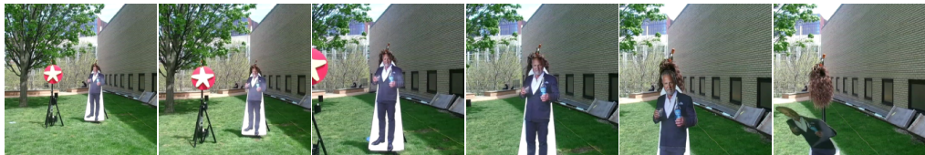
Figure 8: Flex sample real test run: Frames from a test run with text instruction "Fly to the man with a wig". Time increases from left to right. In the last frame, the cardboard cutout is blown off the tripod support by the drone propellers. The wig remains.
