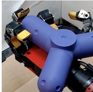
Figure 7: Pose A for the 3-pronged object is approximately 60° offset from Pose B, with any leg pointing straight to the wall.
