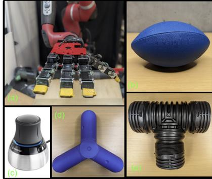
Figure 3: Depiction of our hardware platform and tasks. (a) custom-built 16 DoF robotic hand (c) teleoperation using the 3-D mouse, to interact with the following objects in-hand (b) blue football, (d) 3-pronged valve, (e) T-shaped pipe.
