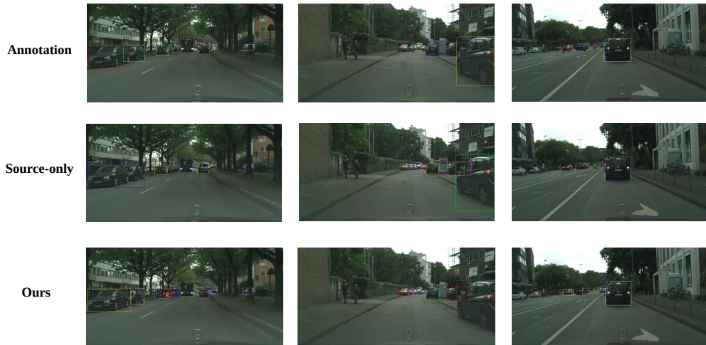
Figure 8: Detection results of adapting the source-only model from SIM10K to Cityscapes.
