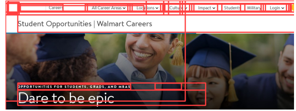
Figure 7: Bounding Box Occlusion Example (parameters chosen to favor occlusion)
