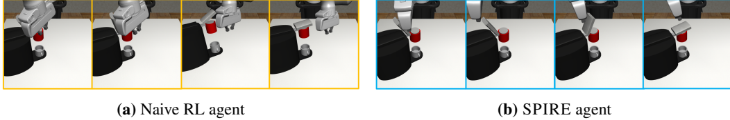
Figure 4: Qualitative comparison. Rollouts of vanilla RL vs our method. The first agent attempts to close the lid by knocking the coffee machine, while our agent follows the demonstrations and closes the lid with fingers.
