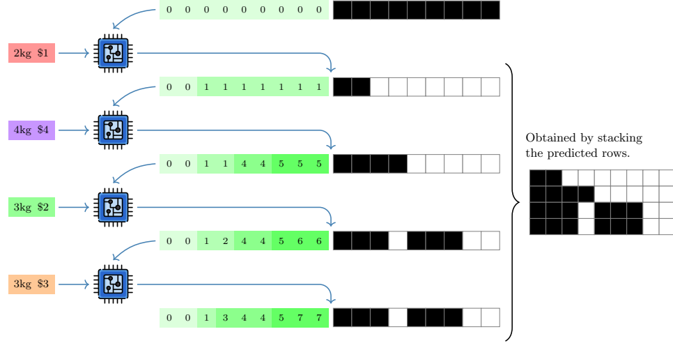
Figure 5: Visualization of the NAR construction process for the Knapsack problem. At each step, the next row of the DP value table and the decision table is predicted from the current latent embeddings. Unlike the standard CLRS-30 approach, where the output is predicted separately using additional node/edge/graph features, our model accumulates the predicted rows of the decision table, which are then passed to the NAR reconstruction.
